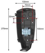
Attach the bracket using fasteners that are appropriate for the type of wall material, drilling pilot holes if necessary. Use the supplied screws only if mounting the bracket directly to a wooden stud. If mounting to another type of wall (hollow, masonry, etc.), use fasteners that are long enough to securely anchor the Wall Connector and can hold at least 36 kg.
