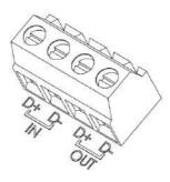
Form a daisy-chained network by connecting the cables from OUT to IN and always from positive to positive and negative to negative between each of the participating Wall Connectors (refer to Example of the Communication Wiring on page 28).
