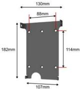
Position the bracket so that the Wall Connector is located at a maximum of 150 cm from floor level. The minimum height is 45 cm if mounting indoors, and 122 cm if mounting outdoors.
